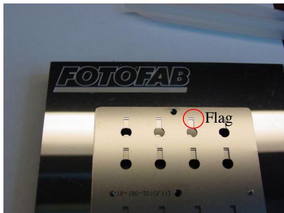
Figure 2-18: Place the top QCM mask.
