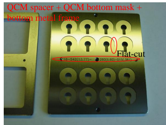
Figure 2-15: QCM spacer and bottom mask.
