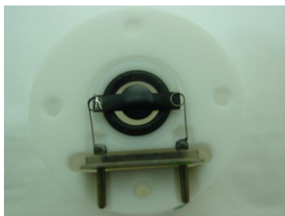
Figure 2-35: Place the EQCM electrode.
