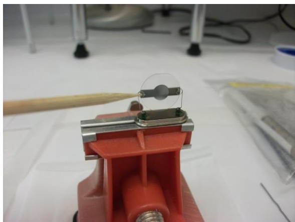
Figure 2-26: Apply Ag epoxy in the connection loop.
