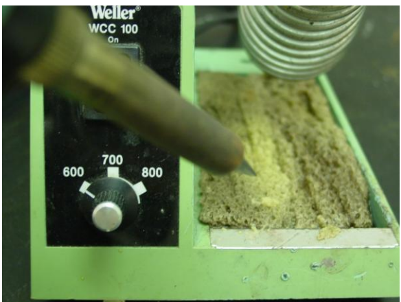
Figure 2-32: Clean the soldering iron.
