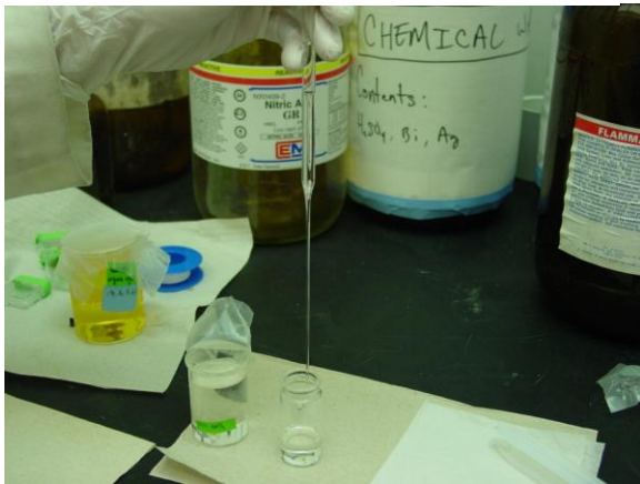
Figure 2-47: Transfer HCl 3 times by Pasteur pipette.
