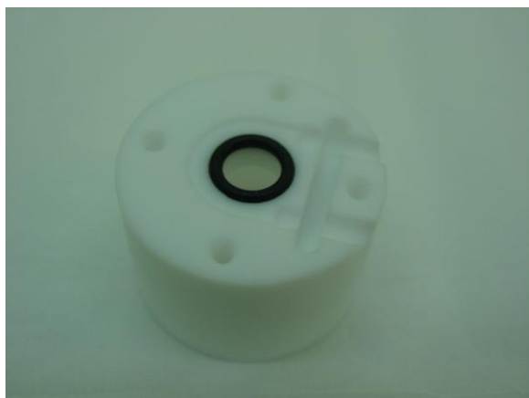
Figure 2-34: Place an o-ring on the EQCM cell.
