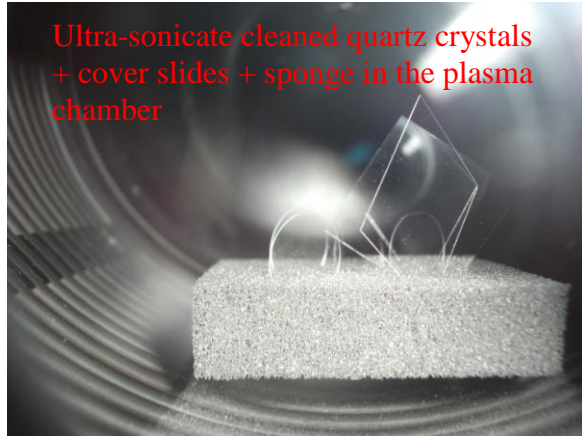
Figure 2-10: Before O 2 plasma cleaning.
