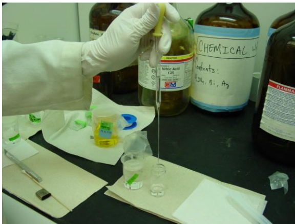
Figure 2-47: Transfer HCl 3 times by Pasteur pipette.
