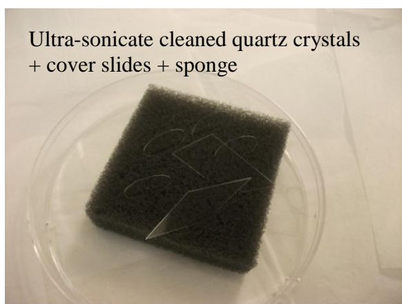
Figure 2-8: Ultra-sonicate cleaned quartz crystals and cover slides stand within the sponge.
