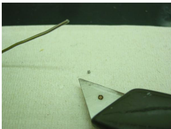
Figure 2-30: Cut a small piece of solder.
