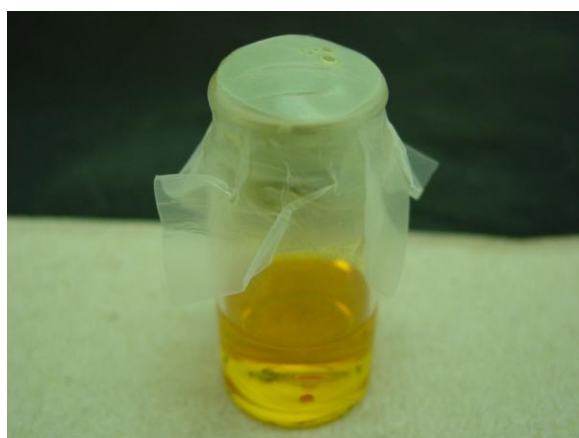
Figure 2-51: Cover the vial with Parafilm.
