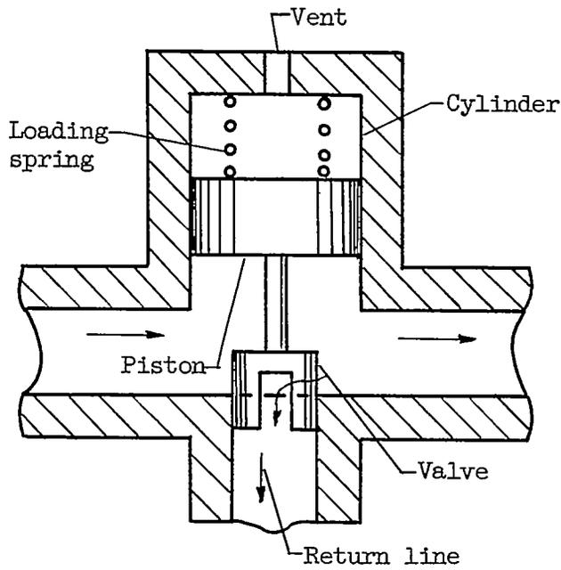
Figure 2. - Schematic drawing of pressure-regulating relief valve.
