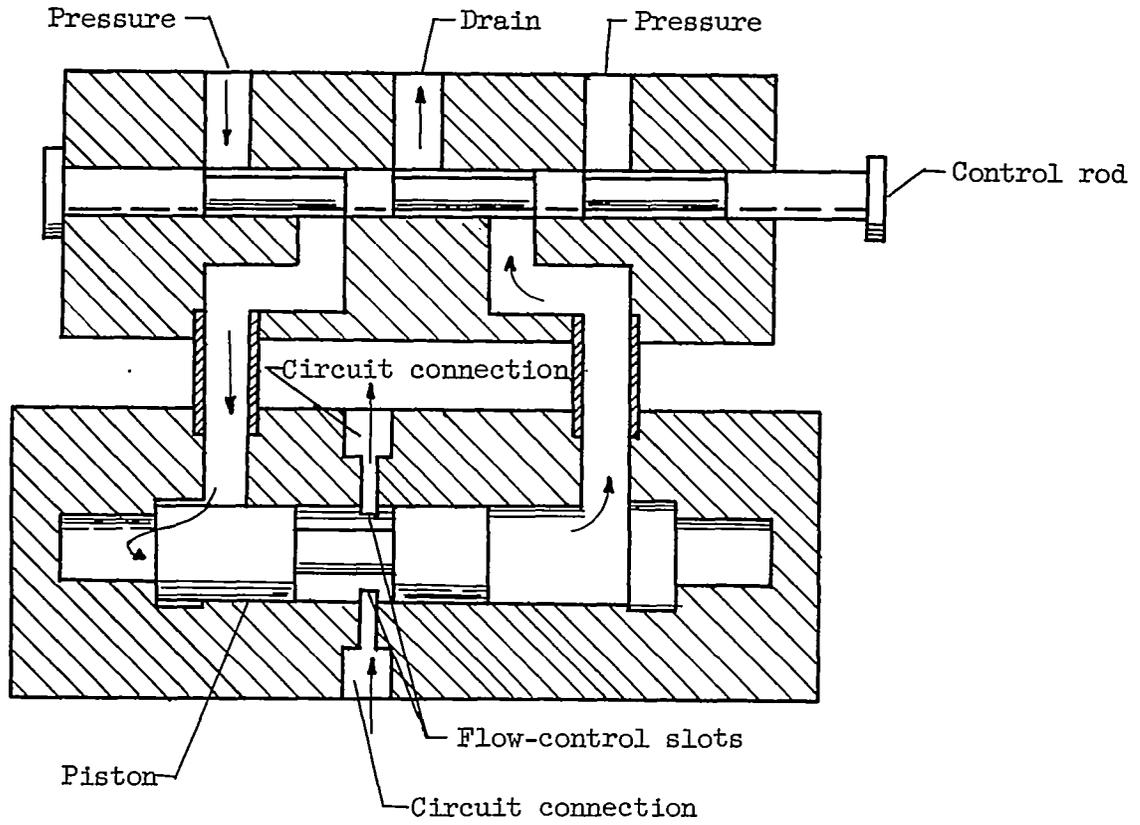
Figure 8. - Schematic drawing of hydraulic switching valve.
