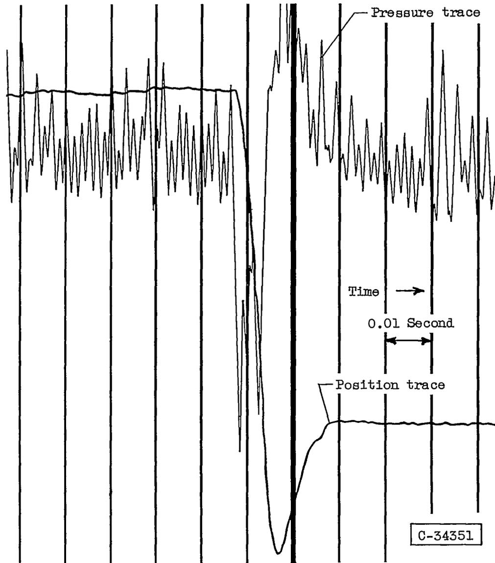
(b) Underdamped case with high distortion.
